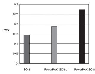
Fig. 4 - Thermal Fatigue Displacement Comparisons
